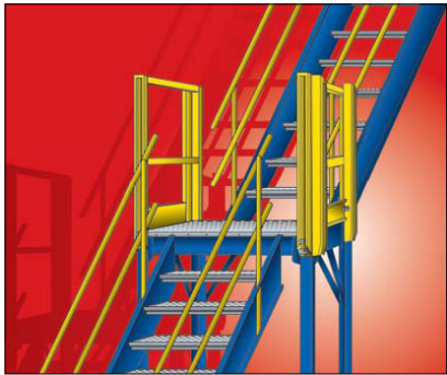
Platform landing is used for straight through passage with stairway proceeding upward.
